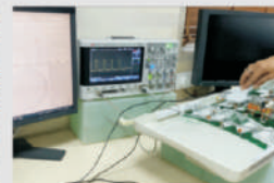
MRI Coil repairs
